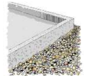
Figure 7. A layer of stones around the slab is a simple way of preventing erosion.
